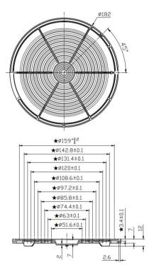
Dimensions with unmarked tolerances refer to GBT14486 tolerance table.
