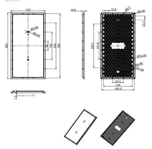
Dimensions with unmarked tolerances refer to GBT14486 tolerance table.
