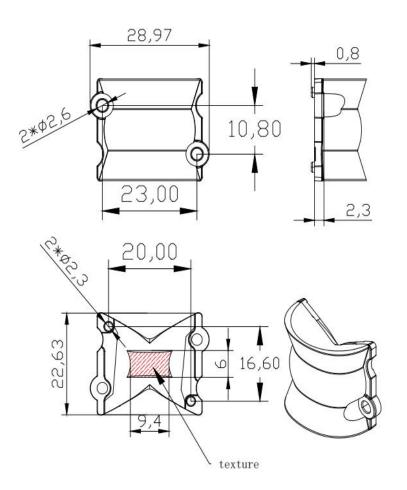
Dimensions with unmarked tolerances refer to GBT14486 tolerance table.
