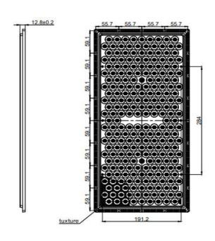
Dimensions with unmarked tolerances refer to GBT14486 tolerance table.
