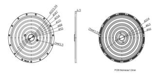
Dimensions with unmarked tolerances refer to GBT14486 tolerance table.
