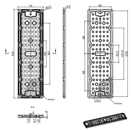
Dimensions with unmarked tolerances refer to GBT14486 tolerance table.
