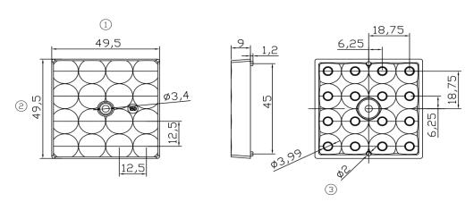
Dimensions with unmarked tolerances refer to GBT14486 tolerance table.
