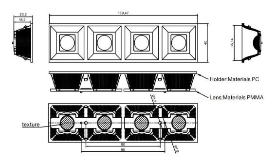
Dimensions with unmarked tolerances refer to GBT14486 tolerance table.
