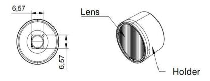
Dimensions with unmarked tolerances refer to GBT14486 tolerance table.
